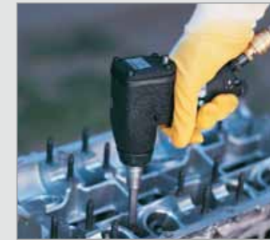
Impact wrenching for repair work
